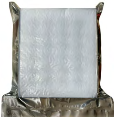
Seal the Tray with Anti-Static Bag
